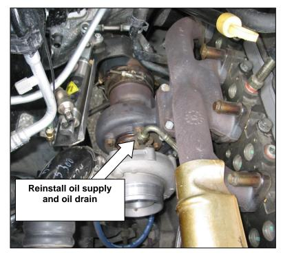
Remove the factory cast exhaust elbow or turbo mount brake using a 7/16" deep socket for the upper V-band clamp and a 10mm deep socket for the lower/rear V-band clamp. Turbo and exhaust manifold can be removed as an assembly if desired. This allows easier access to turbo mounting hardware.
