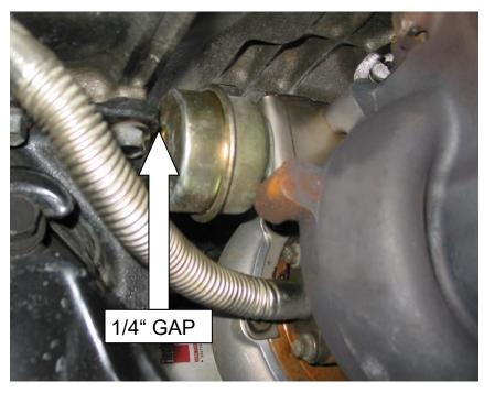
that the compressor outlet elbow does not contact the shock tower.
