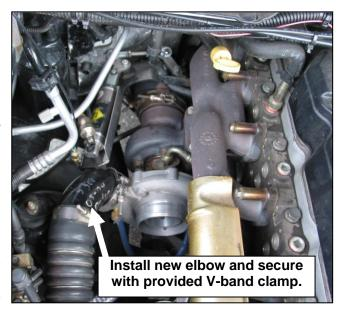
liberal amounts of fresh 15w40 diesel oil into the new turbo while spinning the compressor wheel. Re-install the oil supply line to the top of the turbo.
